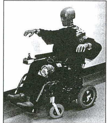
Figure 1 – Hybrid III test dummy seated in P100 test wheelchair
